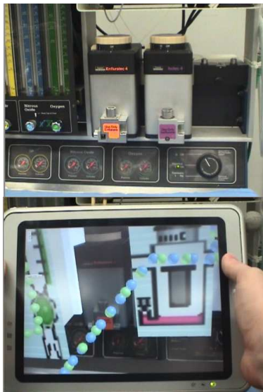
Figure 6. A view of the anesthesia machine vaporizer (top) and the magic lens view of the vaporizer simulation (bottom) shown from the same viewpoint.
