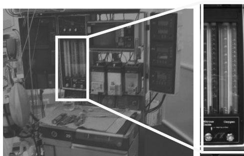
Fig. 4. A magnified view of the gas flowmeters on the real machine.
